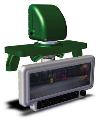
The Driver's Fusion Periscope is a dual waveband device for use on Armoured Fighting Vehicles. The sensor head is capable of being rotated both vertically and horizontally to give the operator a wider field of view. Operating modes include Thermal, Day, Picture In Picture or Fusion: utilising a combination of the Thermal and Day sensors.
